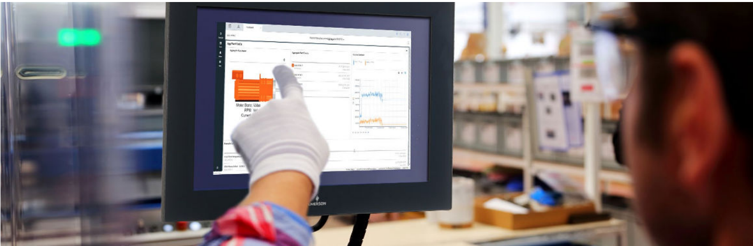
Ten-point projective capacitive touch screens allow for operation with gloves.
