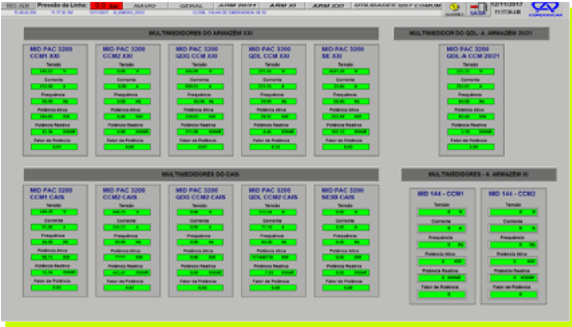
Figure 5: Electrical Quantities - Optimized on a Single Screen
